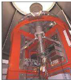
Figure 8: A Typical receiver positioned at the cassegrain focus of one of the VLA-type telescopes
